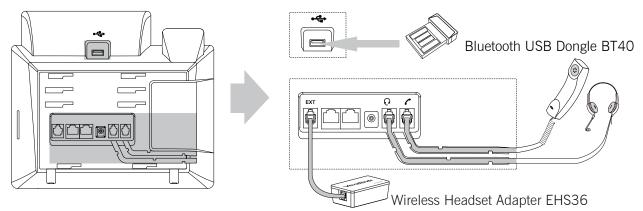
**Note:** The headset, Bluetooth USB dongle BT40 and wireless headset adapter EHS36 should be purchased separately. The EXT port can also be used to connect the expansion module EXP40. For more information on how to use the EHS36, EXP40 and BT40, refer to Yealink EHS36 User Guide, Yealink EXP40 User Guide and Yealink Bluetooth USB Dongle BT40 User Guide.
