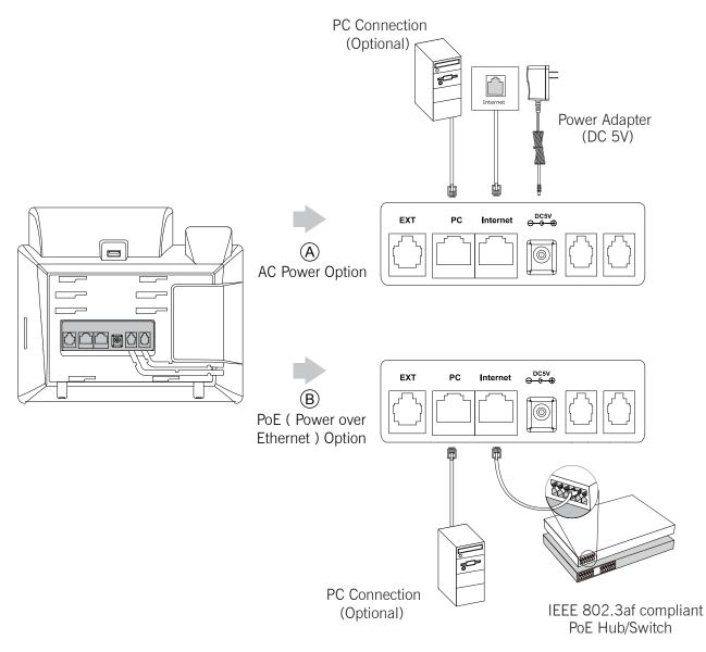
Note: If inline power (PoE) is provided, you don't need to connect the power adapter. Make sure the hub/switch is PoE-compliant.
