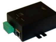
TP-DCDC-1248GD-M (Metal Enclosure)
